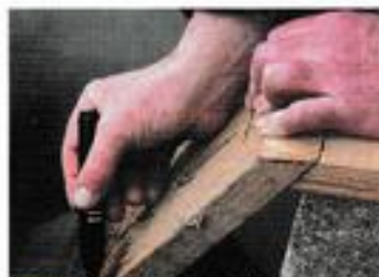
STEP 3 Fit the two pieces together and mark the second piece about 25mm below the water surface and cut through at 90 degrees.
